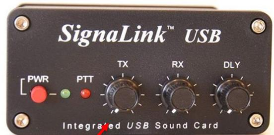
Adjust for TX Level on Signalink
