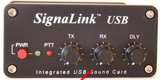
Adjust for RX Level on Signalink
